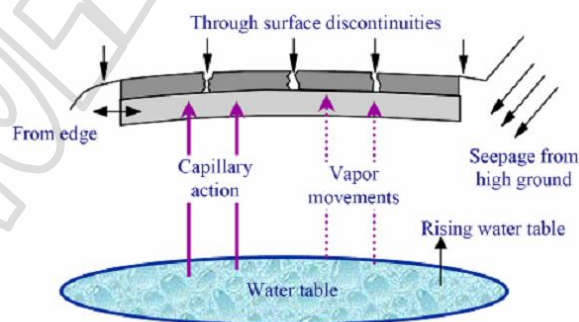
Figure 1. Sources of moisture in pavement systems [2].
