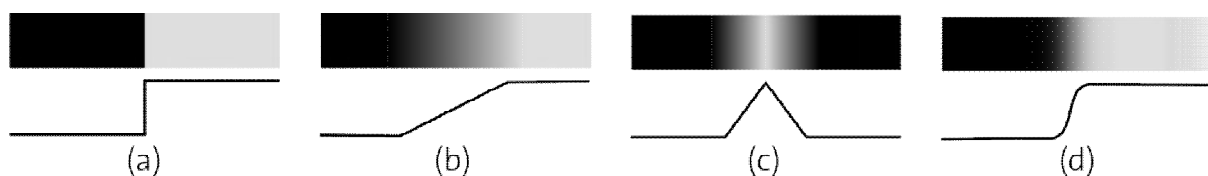
Figure 1 - The most common edge models (a) step or ideal edge, (b) ramp, (c) roof edge, and (d) the real edge
